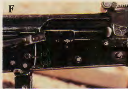
F: Receiver with selector lever in safe position. "AB" is full-auto and "OA" is semiautomatic fire.
